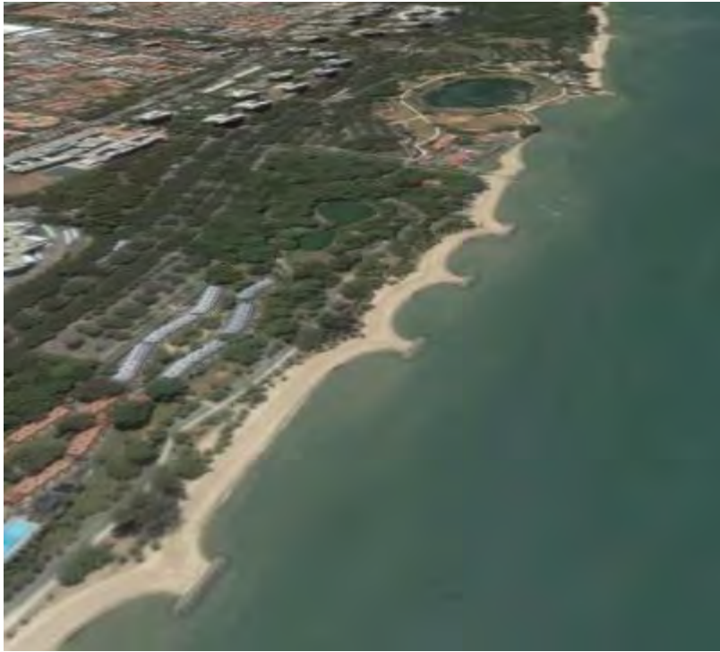
Use of headlands to stop erosion on the south coast of Singapore since 1971
