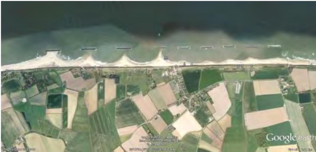
**Breakwater scheme at Sea Palling, Norfolk, UK**
