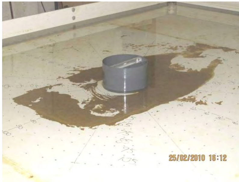
View from seaward side of cylindrical island after 77 hours of wave action
