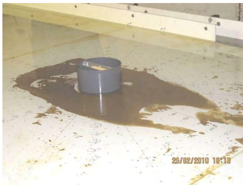
View from landward side of cylindrical island after 77 hours of wave action
