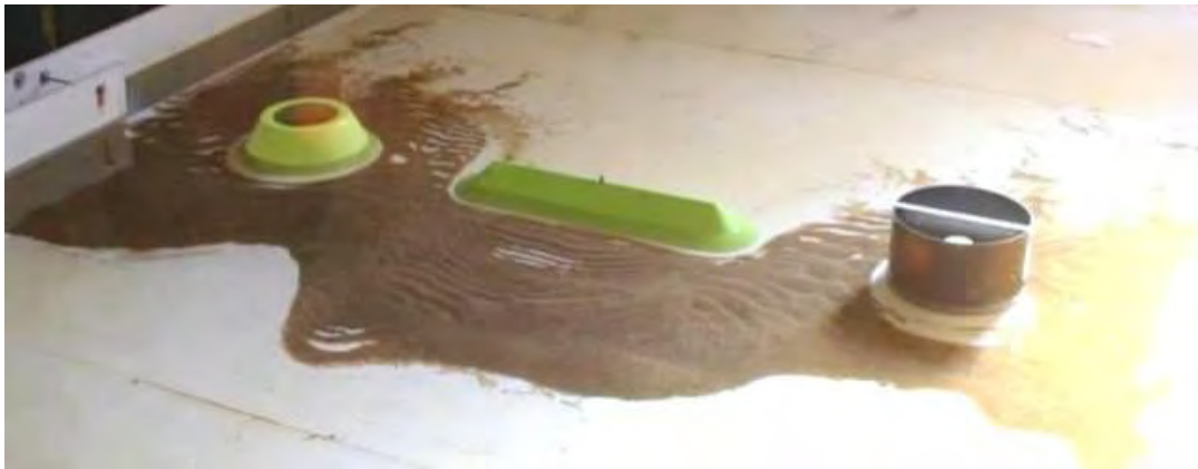
Simultaneous test of alternative headland shapes – 2 hours of wave action
