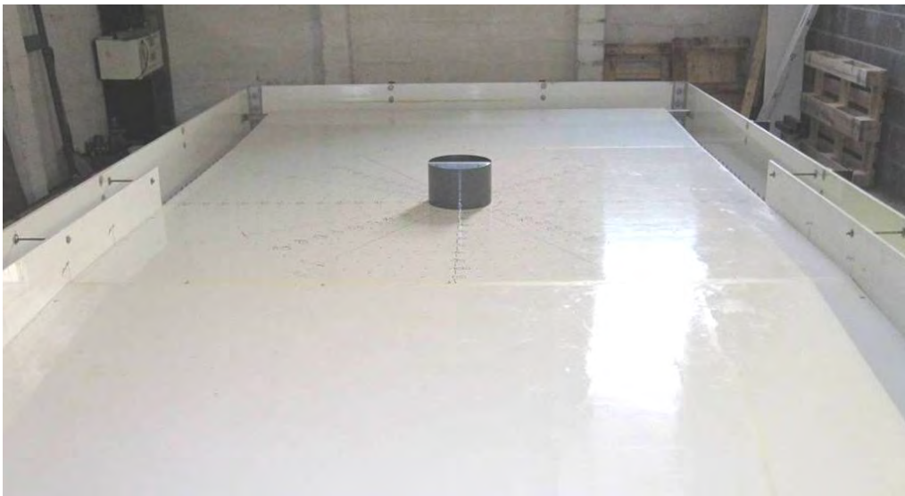
Test tank and cylinder viewed from wave machine end
